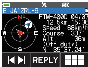
Example of display when an APRS signal is received
