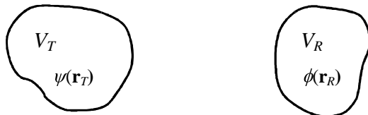
Fig. 1. Illustration of transmitting ( V_T ) and receiving ( V_R ) volumes, with associated source ( \psi(\mathbf{r}_T) ) and wave ( \phi(\mathbf{r}_R) ), functions
