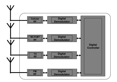
Figure 1: Traditional Radio Frequency Architecture
