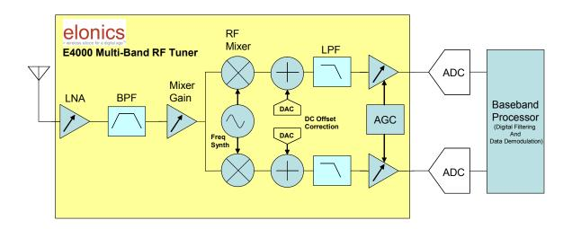
Figure 9: Multi-Band Radio Receiver Solution
