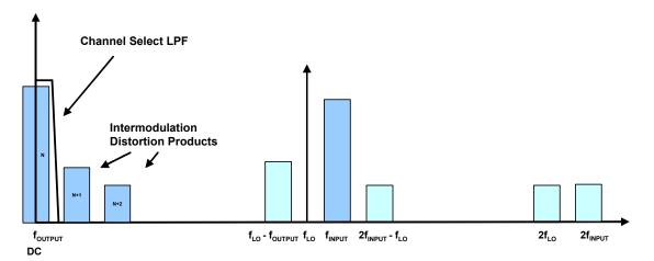
Figure 8: Mixer Output Spectrum
