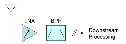
Figure 5: RF LNA and Filter
