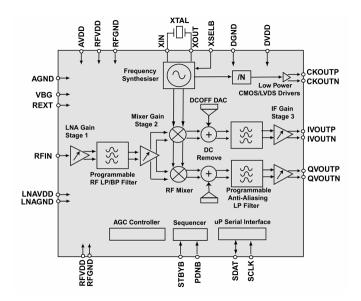
Figure 4: E4000 RF Tuner Block Diagram
