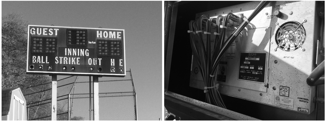
Figure 2: FairPlay 710 scoreboard and internal processor box.
