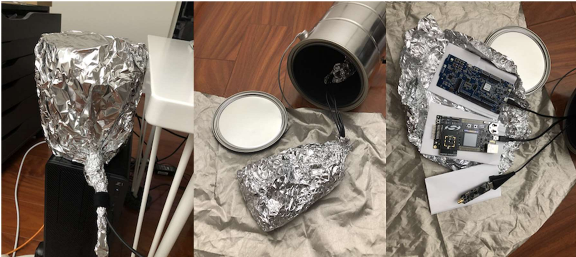
Figure 7. Baked-potato style Faraday cage
