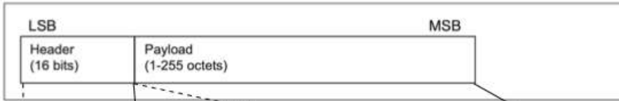
Figure 2.4: Advertising physical channel PDU
