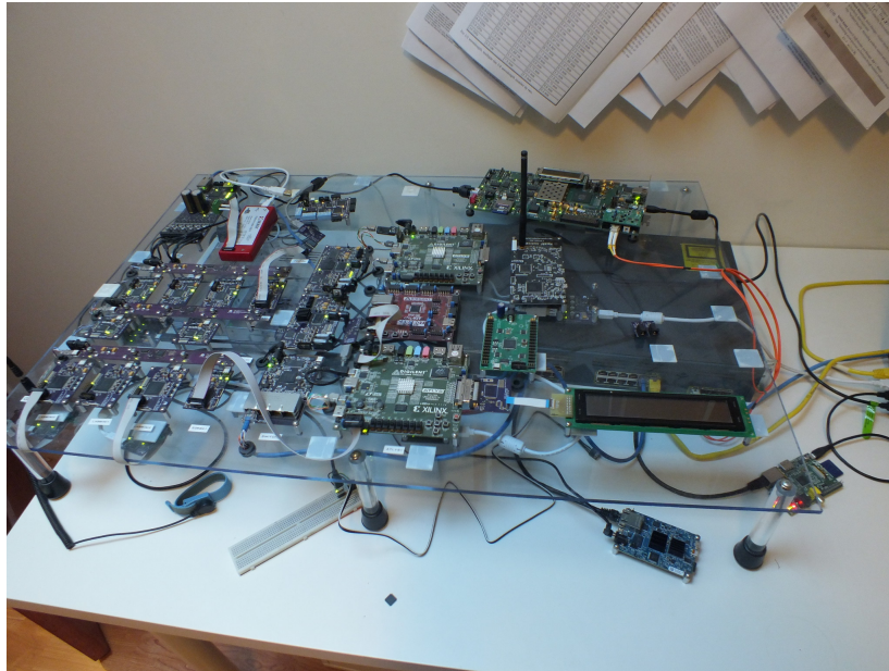
Figure 4.4: Large FPGA cluster on desk
