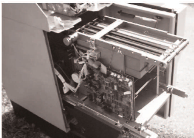
Fig. 4: Rails extended, electronics and cash handler visible
