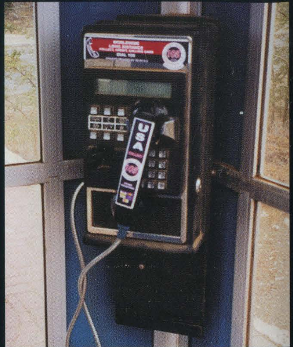
Looking closer, we can see that this is a card-only phone with the coin return and coin box missing, which is why it seems so squat.
