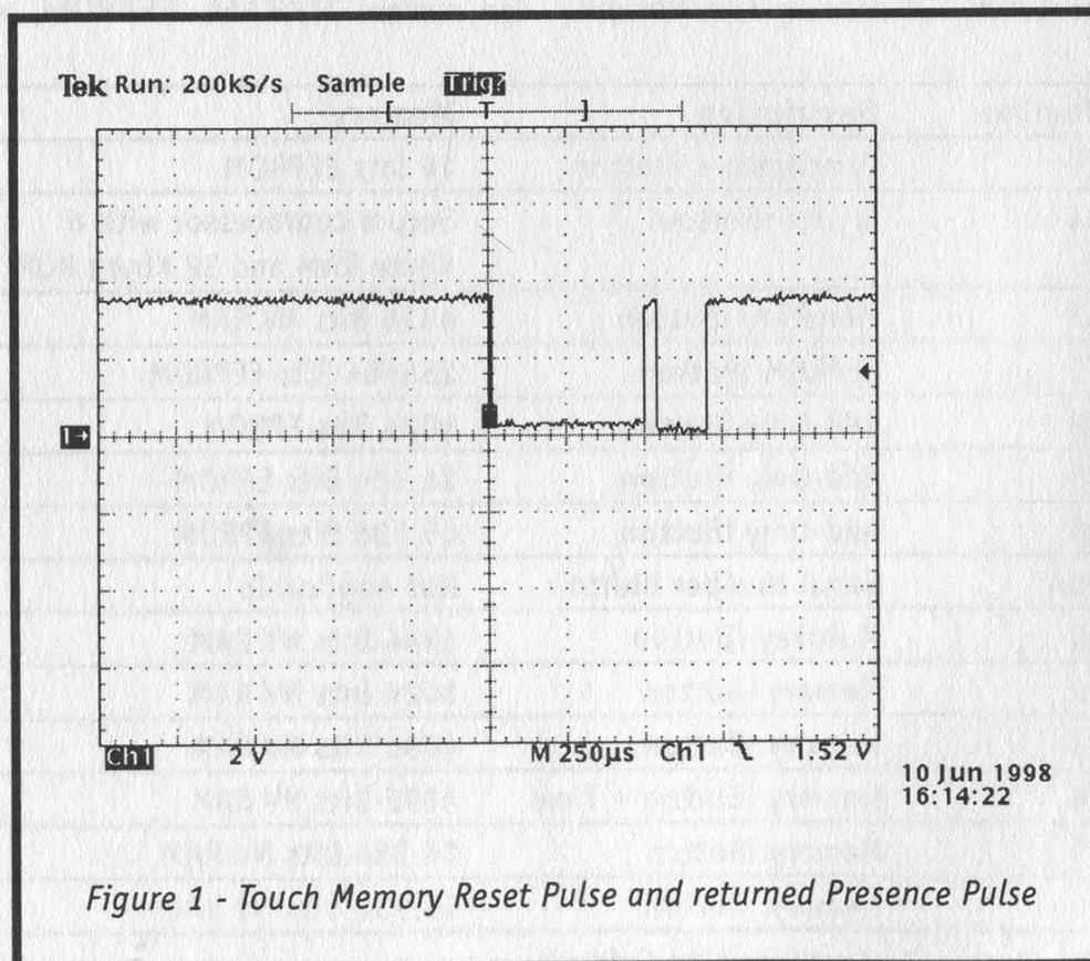
Figure 1 - Touch Memory Reset Pulse and returned Presence Pulse
