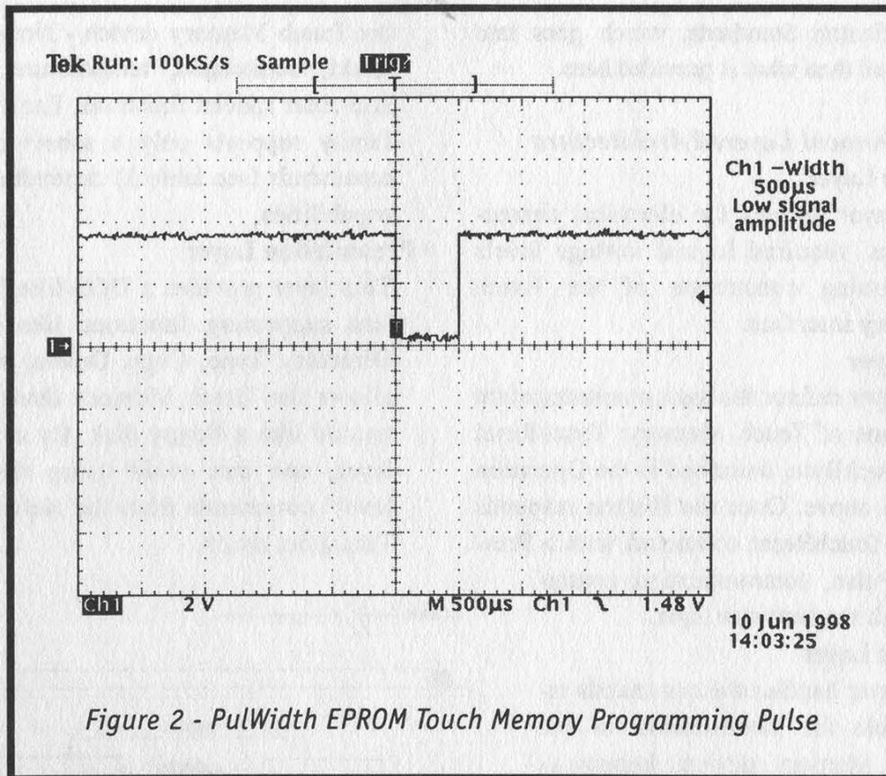
Figure 2 - PulWidth EPROM Touch Memory Programming Pulse
