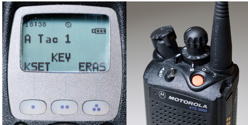
Figure 6: XTS5000 in “Encrypted” Mode
