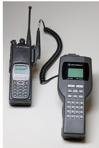
Figure 4: Motorola KVL3000 Keyloader with XTS5000 Radio
