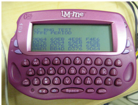
Figure 7: Girltech IMME, with modified firmware
