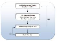
Figure 6.8: Loop structure of GetAsyncKeyState and GetForegroundWindow in keylogger
