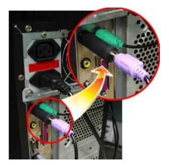
Figure 6.2: Hardware Keylogger
