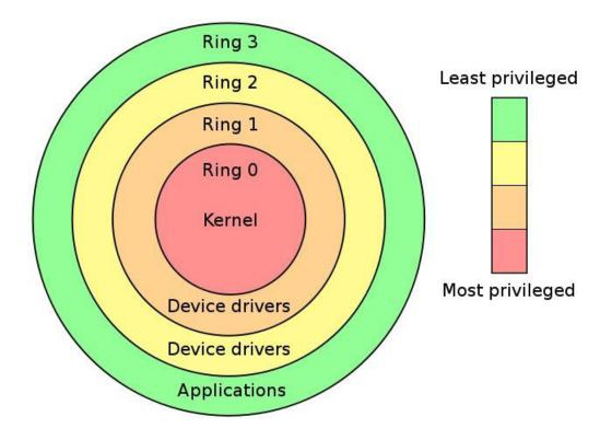
Figure 2.12: Figure of protection rings. Rings are mechanisms to protect data and functionality from faults and malicious behavior. (Image source: Wikipedia)
