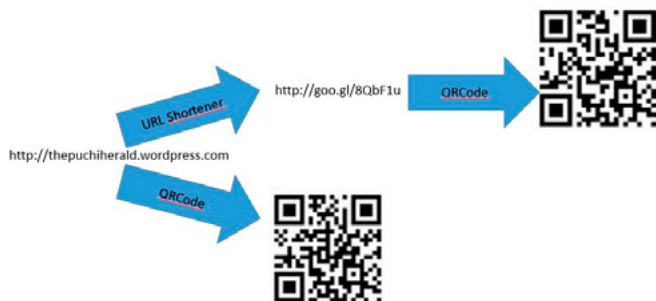
Figure 3. Qrcode can be generated from an URL or the shorter version. When using a URL Shortener service we loose readability of the URL address thous is easier to be redirected to a fake site
