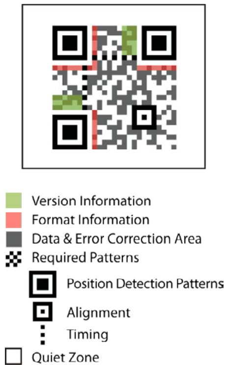
Figure 1. Anatomy of a QR Code Courtesy DENSO Wave, Inc.
