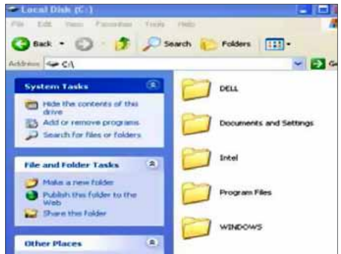
Figure 6. A screen capture of the folder list of C drive showing Hacker Defender rootkit folder is hidden
