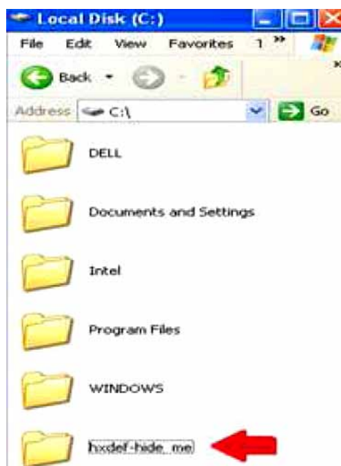
Figure 4. A display window of the folders on the C drive. The red arrow points to the folder with hxdef , which will be hidden by Hacker Defender
