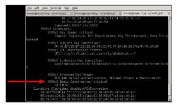
**Figure 1.** The field CA=FALSE must be specified to restrict generating new certificates
