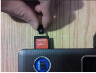
**Figure 3.** The adapter for uSD card to read it from pc.
