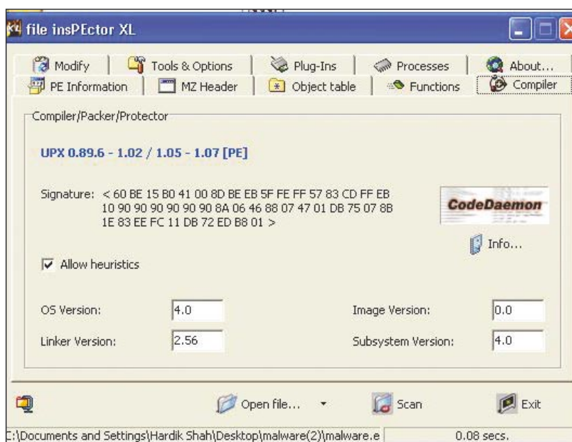
Figure 1. File inspector showing the packer as UPX
