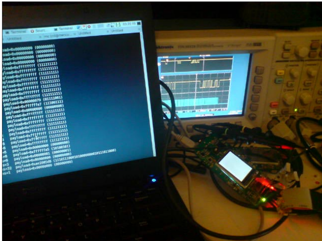
Figure 11. Practical low-level access to embedded system prototype hardware using JTAG/SWD debug port
