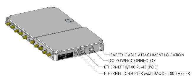
Figure 9 - xBR V4 Connections
