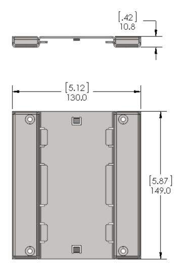
Figure 2 - Quick Release Adapter
