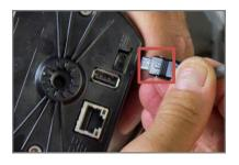
Figure 10.6 – Plugging in the Ethernet and Power Lead
