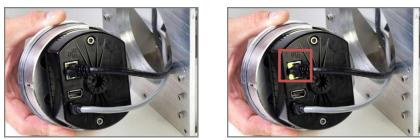
Figure 10.7 – Ethernet Indicator Lights
