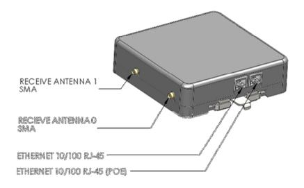
Figure 5 – xBR Connections
