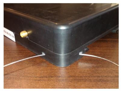
Figure 4 - Safety cable attachment point
