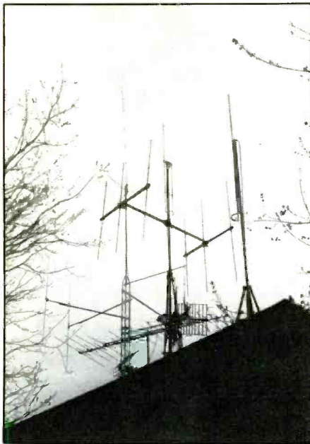
The author's AS-756/TRC military surplus antenna is a dual three element yagi that will operate between 30 and 100 MHz.
