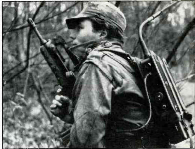
The French military TRC559 military manpack transceiver operates with NBFM with channels spaced 25 kHz apart between 30 to 80 MHz.
