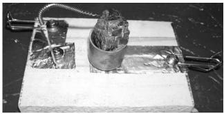
That is the heart of a crystal radio setup, made from a copper pipe cap, a piece of Galena, and some other assorted parts. The cats-whisker was made from the spring of a discarded Bic lighter. Add a tuning coil made from copper wire and some more scrap parts like this:
