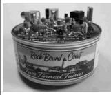
These days you don't need CW to get a ham ticket, but for less than \$100 build a CW QRP rig set-up that will fit in a field jacket pocket. A fellow ham
