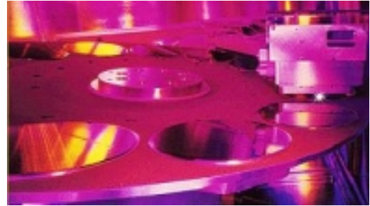
A wafer handling tray in ion implantation
