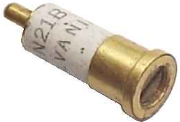
Picture 2. Early point contact diode with adjustable screw
