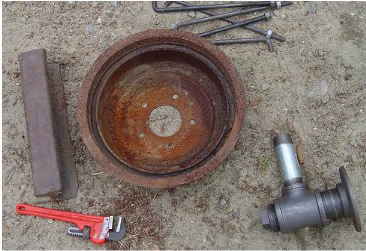
This brake drum forge is made from a large truck brake drum, with pipe parts for the blower pipe.
