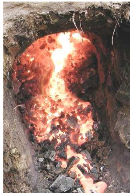
Base of smelter. Note air pipes, which supply fire with oxygen. Molten metal, in base of smelter.
