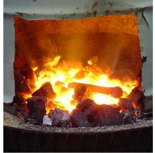
This brake drum forge is made from a large truck brake drum, with pipe parts for the blower pipe.
