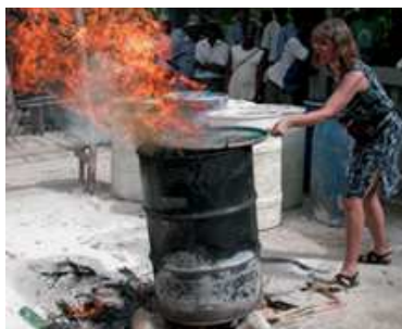
Making charcoal in a 55 gallon drum, and view of completed charcoal.
