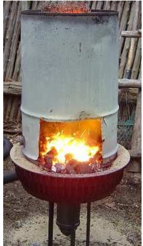
Here is the completed forge, and the forge in use, with a 30 gallon drum, used as a wind shield.
