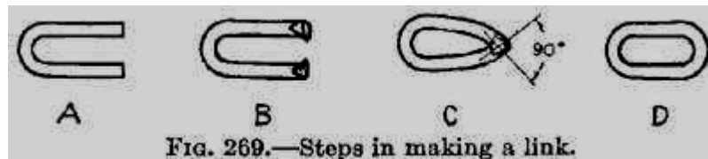
Fig. 269.-Steps in making a link.
