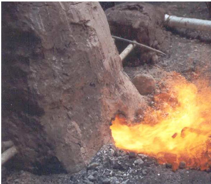
Base of smelter. Note air pipes, which supply fire with oxygen. Molten metal, in base of smelter.
