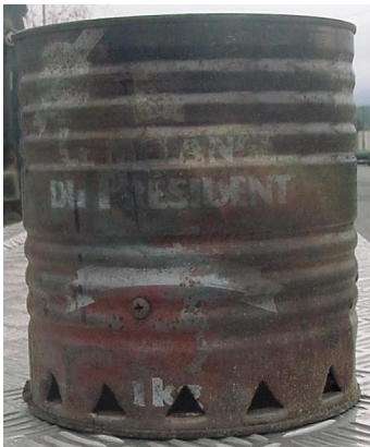
Camp Can Stove: Any large metal can may be fashioned into a useful camp cooker.
