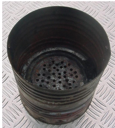
Camp Can Stove: Any large metal can may be fashioned into a useful camp cooker.
