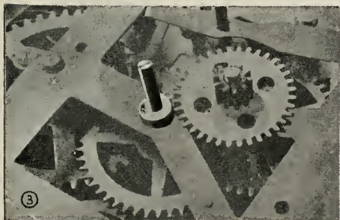
PINION IS RETURNED TO ORIGINAL POSITION
