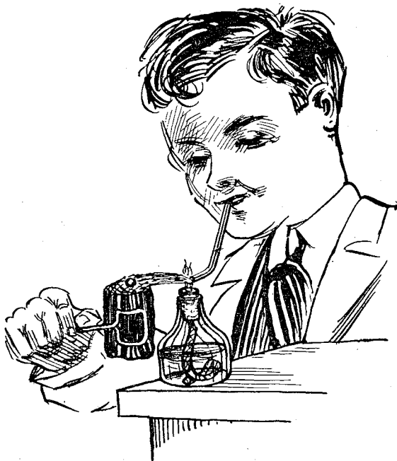
FIG. 126.—How to Heat Antimony with a Blow-Pipe.
