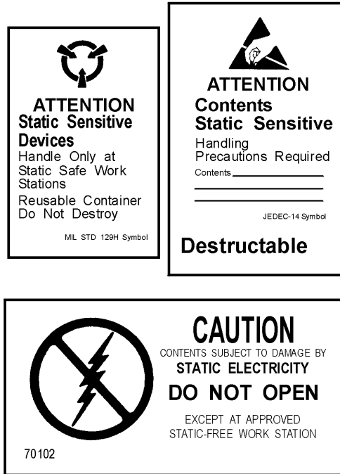
Figure 2-5.—Warning symbols for ESDS devices.
