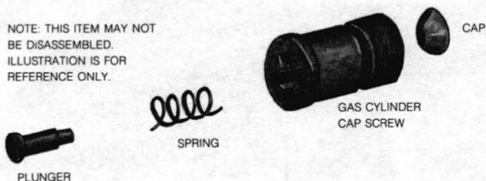
Figure 44. Gas cylinder cap screw, current type — exploded view.
