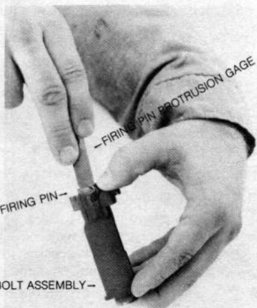
Figure 47. Gaging firing pin protrusion.
