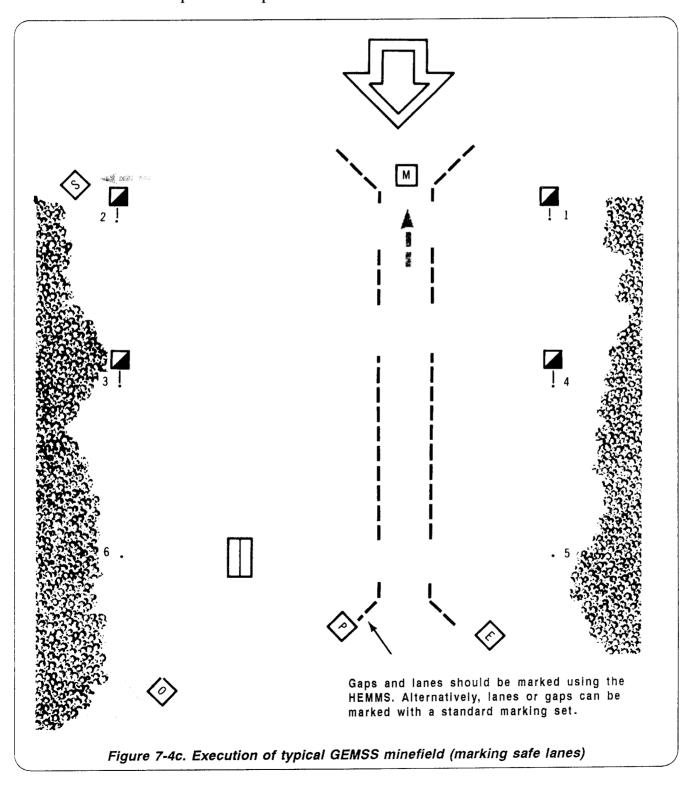
Marking the minefield (Figure 7-4d). The marking party marks the minefield boundaries. The marking party is assisted by members of the siting and emplacement parties as needed. Fences are emplaced 60 meters beyond the
