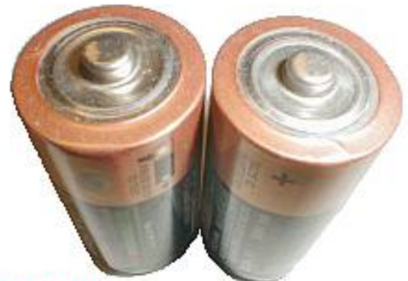
Picture 2. Oxide spots on new batteries
