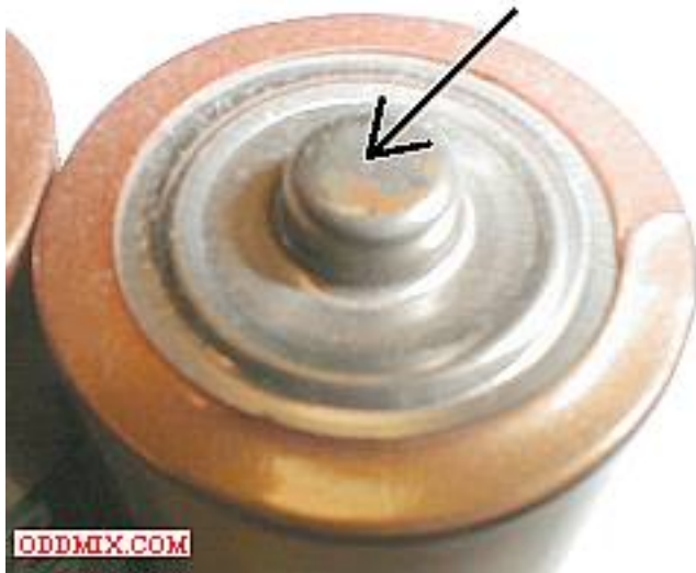
Picture 1. Red oxide spots on battery
