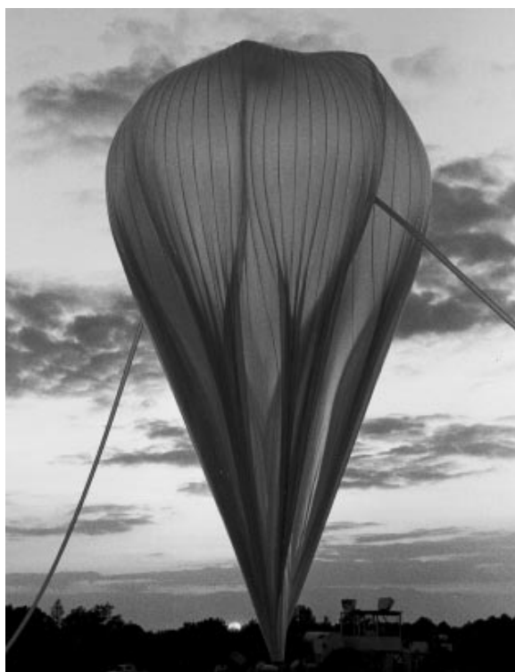
Final inflation of an instrument-carrying helium balloon before launch from Palestine, TX
