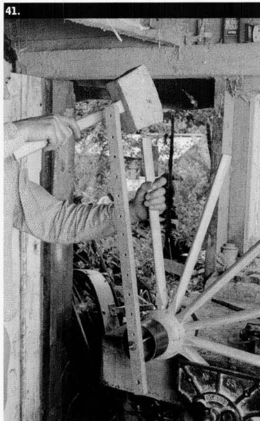
41. The whalebone gauge in use, here a light wheel is held in a joiner's vice.
