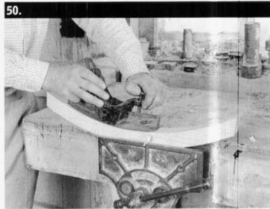
Cleaning up the belly of a felloe with a compass plane.
