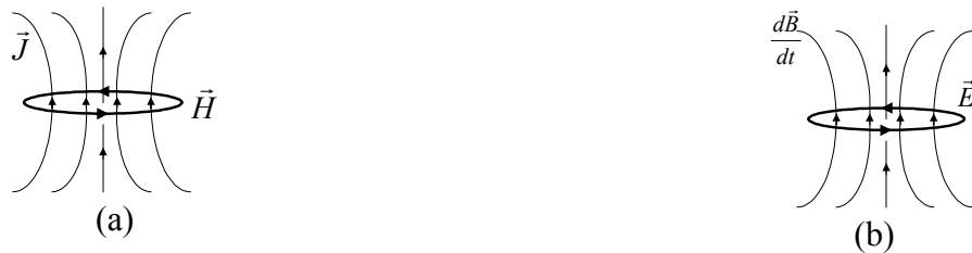
Figure 1. Figures illustrating use of Maxwell's equations. (a) Ampere's law. (b) Faraday's law.
