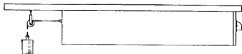
The Rope and Weight Attached to the Back End of the Drawer Pulls It Closed
