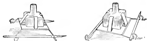
Tilting Stand for an Ordinary Ink Bottle to Give Access for a Small Supply of Ink
