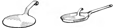
A Metal Plate for Use in an Ordinary Frying Pan to Cook Eggs without Scorching Them
