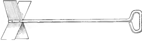
The Chopper Consists of a Rod Handle to Which Blades are Attached by Riveting or Welding
