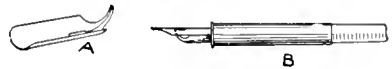
The Space between the Pens Forms the Fountain, Which is Sufficient for Considerable Writing
