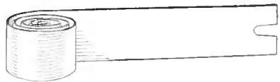
A Strip of Tin Shaped to Take the Place of a Rivet Set
