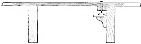
Push Button on Joist
