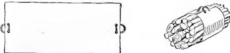
The Ropes at the Ends of the Sack Make a Handle to Carry It Like a Grip
