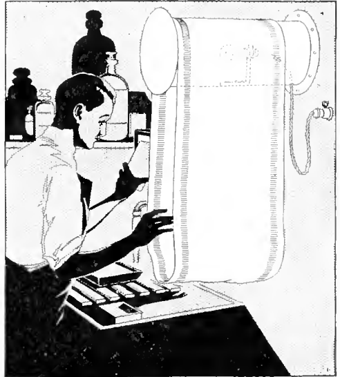
An Electric Globe Makes Heat in the Spool for Drying a Portion of the Towel
