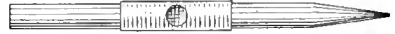
A Torch Made of Glass and Rubber Tubing, to be Used on an Ordinary Gas Jet
