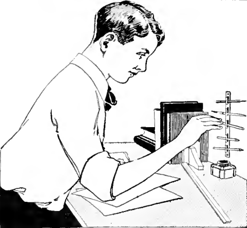
A Strip of Sheet Metal Cut and Clips Formed to Make a Pencil Rack
