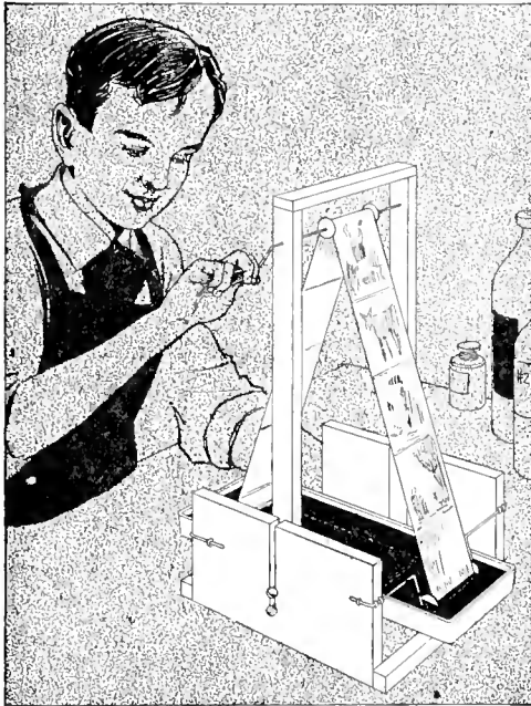
Developing a Roll Film in a Tray with a Machine That Drives the Film around Rollers and through the Developing Liquid by Turning a Crank
