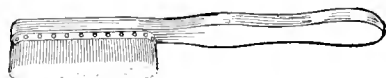
Brush Made of Strip of Upholsterers' Haircloth with the Warp Removed and Fastened to a Handle
