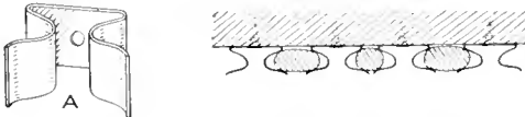
The Clips can be Set So That They will Grip Any Size Tool Handle
