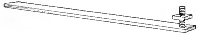
The Nut is Set to the Thickness of the Glass and Used to Break Pieces Away
