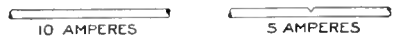
The Amperes of a Fuse Reduced by Making a Nick in the Lead Wire
