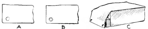
The Hooks Prevent the Covers from Slipping Off the Sleeper and Keep Them Straight on the Bed
