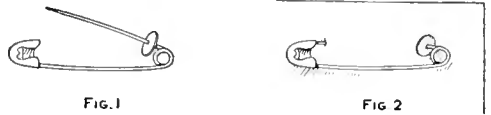
The Small Disk on the Pin Prevents the Goods from Becoming Tangled in the Coil
