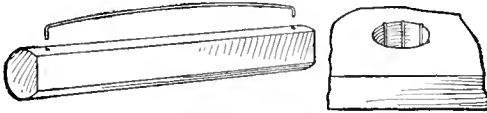
The Spring Wire will Hold the Stop at Any Desired Position for Height
