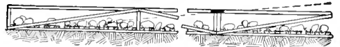
The Series of Platforms Make a Good Small-Boat Landing on a Slanting Beach
