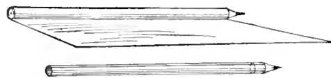
A Stub of a Pencil can be Easily Held in the Tube for Writing
