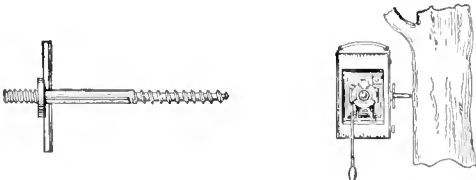
Substitute for a Camera Tripod That can be Carried in the Pocket Like a Pencil
