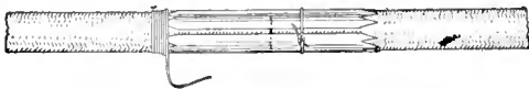
The Repair on a Whip Made with a Notched Ferrule and a Waxed Thread
