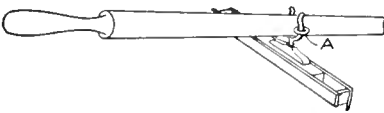
The Screweye in Position on the Oar and over One Prong of the Oarlock
