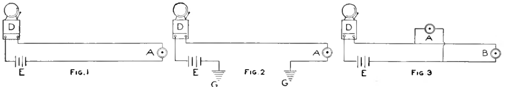
Wiring Diagrams for a Single Bell
