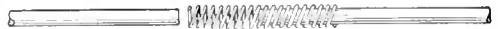
A Coil Spring Used for Splicing Sash Cords or Small Round Belts
