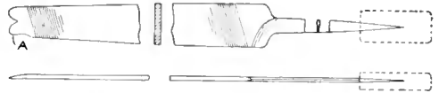
A Tool Made of a File Combining Several Tools Which are Used by a Draftsman
