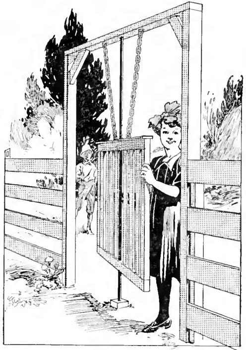
The Gate will Swing in Either Direction and Come to a Rest Where It Closes the Opening
