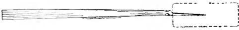
A Very Small Eraser can be Held on the Point and Used for Delicate Erasures
