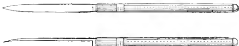
One of the Nibs on the Ruling Pen Sharpened and Used as an Eraser
