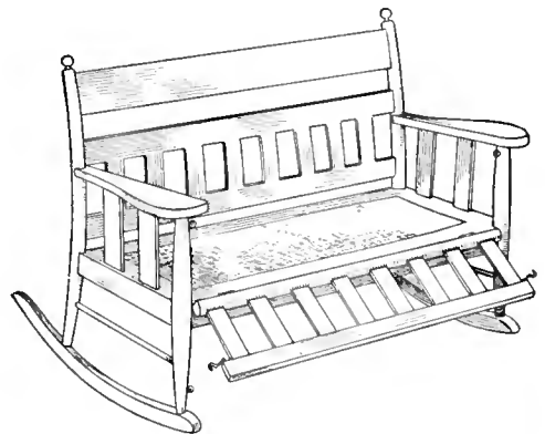
A Settee Rocker with a Front Attachment to Make It into a Cradle When Desired
