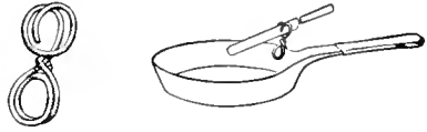
The Shape of the Clip and Manner of Attaching It to a Frying Pan
