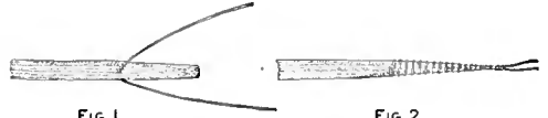
The Wire Prevents the Lace from Raveling and Makes a Tip for Easily Entering the Eyelets
