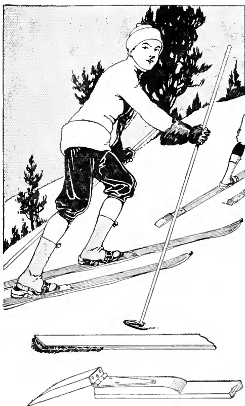
Two Methods of Making an Attachment to Prevent the Backward Thrust of a Ski
