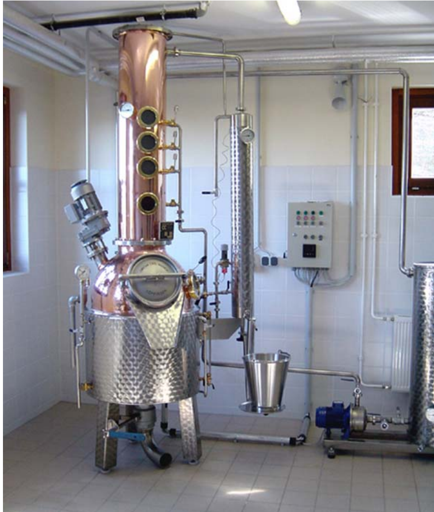
Figure 12. An electrically heated still with rectification column directly mounted above the pot. (Figure courtesy of Christian Carl, Ing. GmbH)
