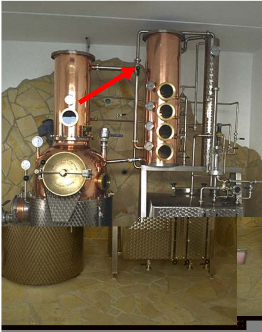
Figure 13. A steam fired still with the rectification column set to the side. This configuration allows a complete bypassing of the column to approximate an alambic or Rayleigh distillation. This same bypass configuration would be appropriate for the production of gins and flavored vodkas. The red arrow indicates the valve allowing the bypass. (Figure courtesy of Christian Carl, Ing. GmbH)
