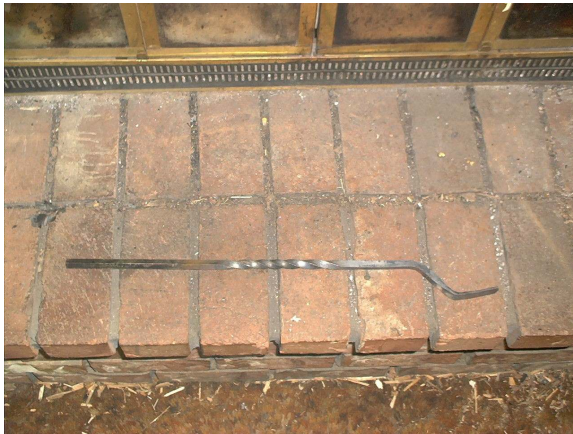
A shovel handle ready to be fitted with a scoop.
