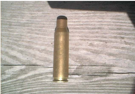
Case denting was cured with a little work on the receiver cover.
