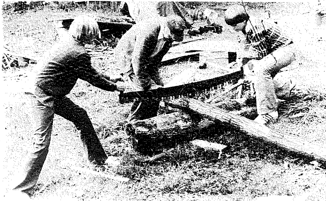
PLATE 262 Roger Fountain and Bill Taylor saw off a 2'-long piece of locust while Clyde holds the log. This piece will form the two wagon axles.
