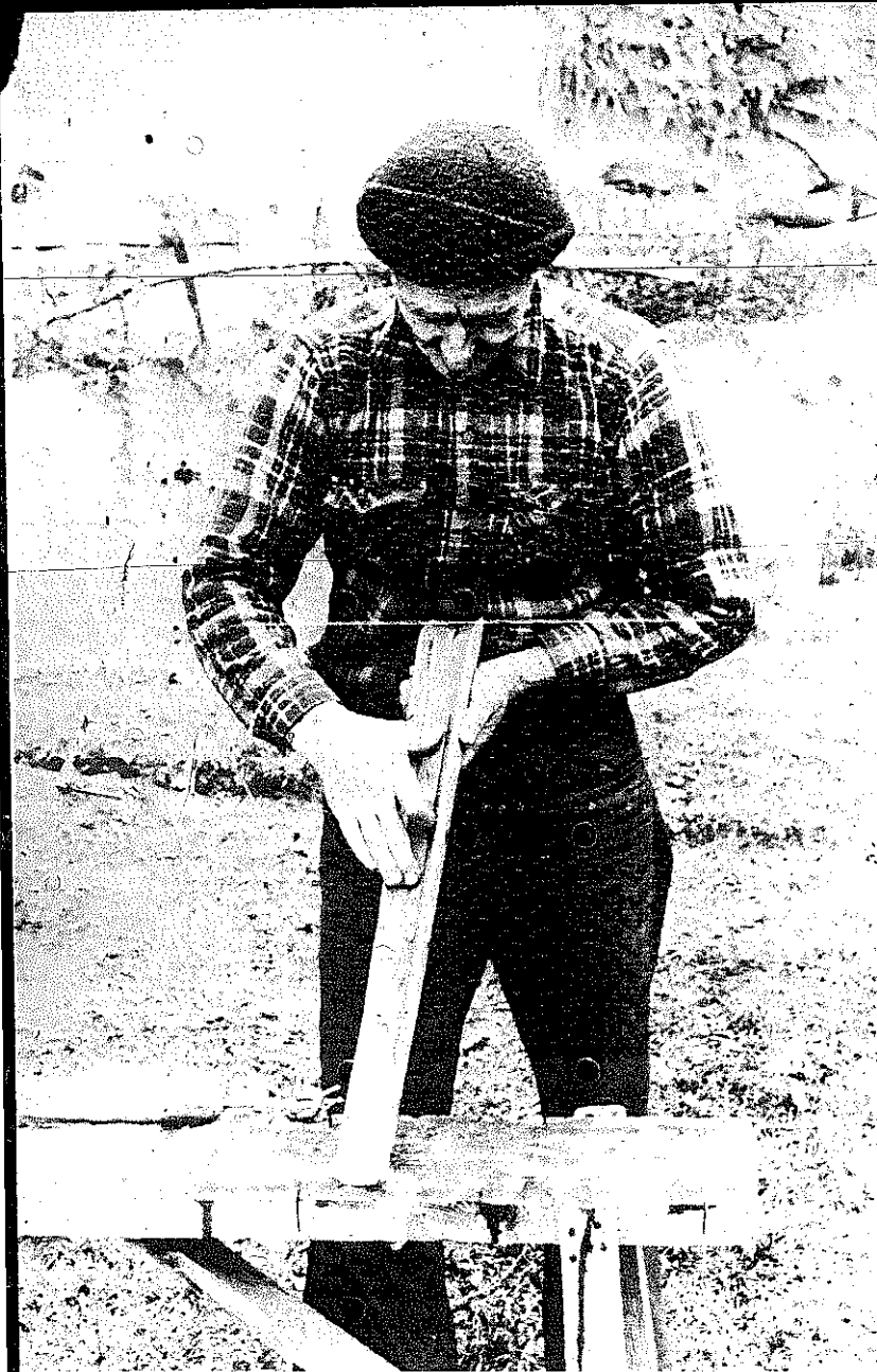
PLATE 27 Leonard rasps the fingerboard for precision fitting. Special attention is given to areas where the fingerboard meets the banjo head and on the sides where the fingerboard meets the neck.
