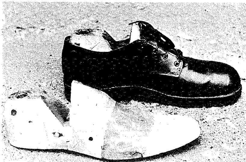
PLATE 110 The wooden lasts Ernest uses to make shoes for himself. Metal lasts are used only for repair work—not for making shoes.
