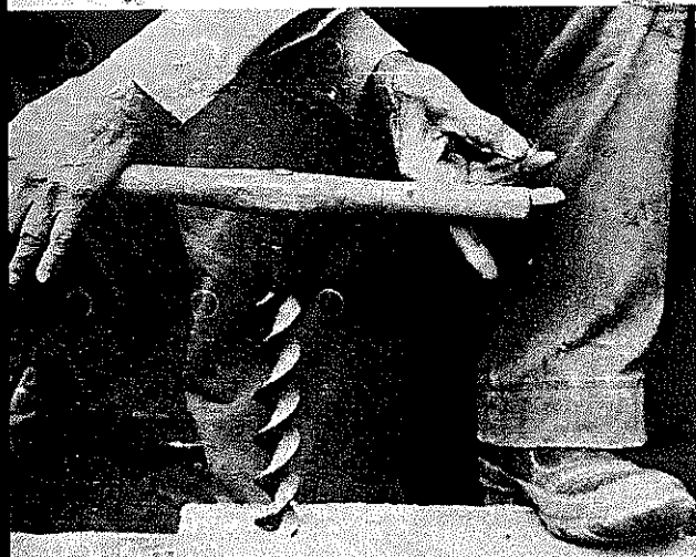
PLATE 35 Bill Lamb, with an auger, shows how one can get a "double lick" by crossing the hands thus allowing one complete revolution of the tool.
