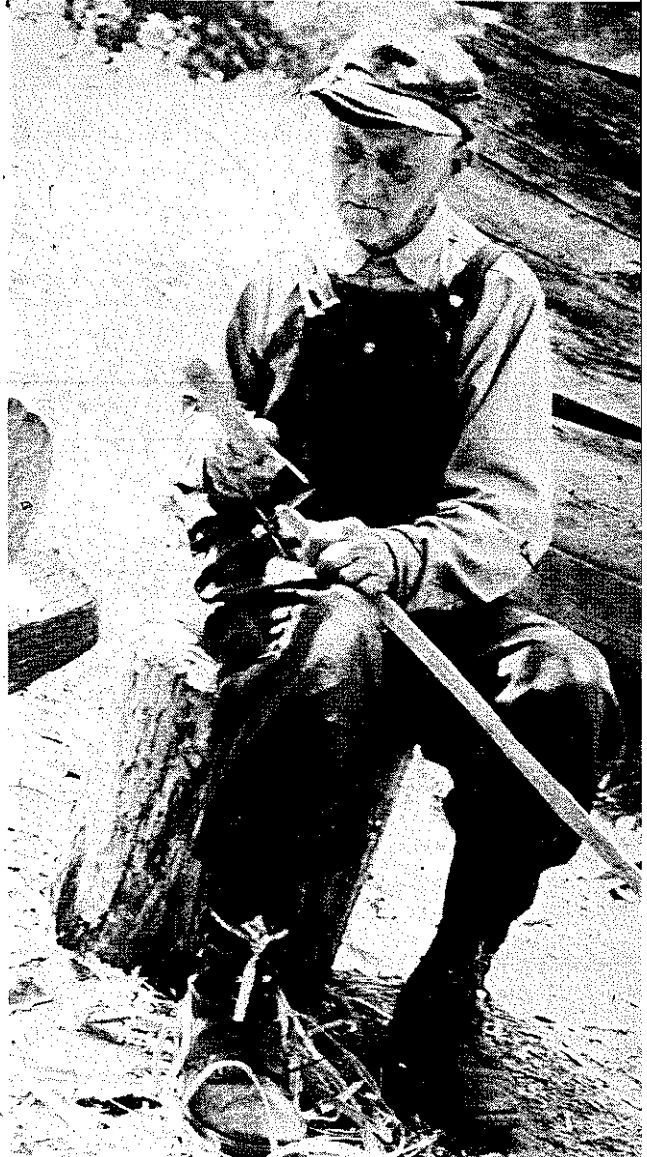
PLATE 154 The actual process of making the splits now begins. Beginning at the butt end of one of the prepared eighths, split it exactly in half parallel to the grain of the wood, or "bastard fashion." Some split them off perpendicular to the grain ("board fashion"), but most prefer Lon's method. The split can be started by driving a pocket knife blade into the bolt with a piece of scrap wood.
