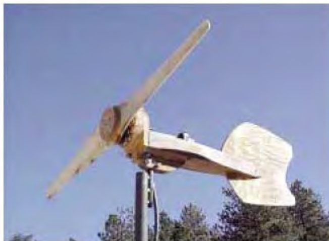
The next generation—the WoodAx is for permanent installation, and produces upwards of 300 watts in 30 mph winds.
