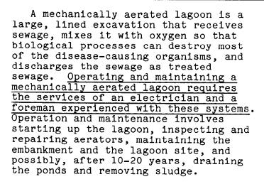
Correct operation and maintenance is important because a neglected lagoon will produce foul odors, become a breeding place for flies and mosquitoes, and require costly repairs. This technical note describes how to operate and maintain a mechanically areated lagoon.
