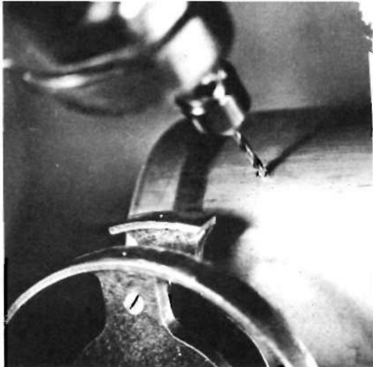
Drill mirror mount holes 1-2" from end of main tube. Mirror must be mounted squarely in the tube.
