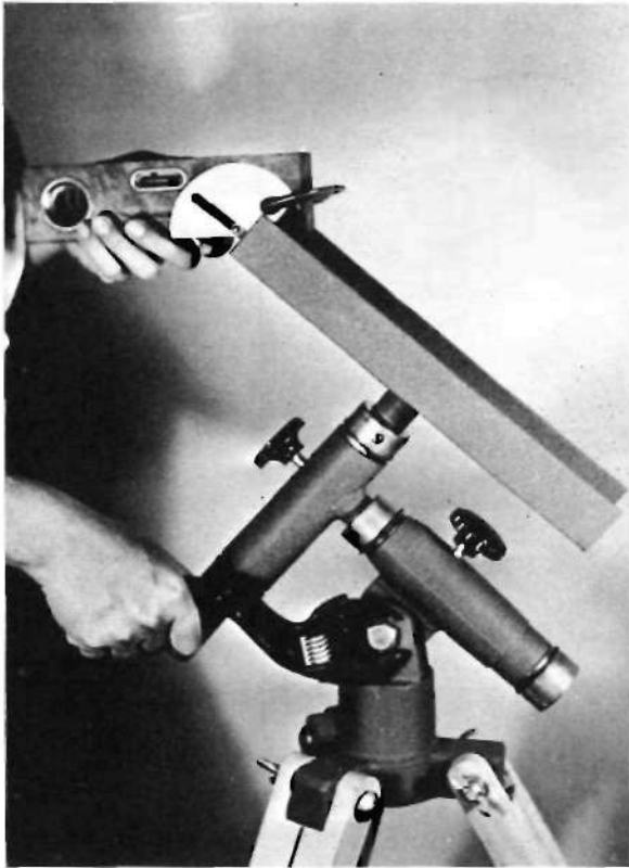
Check your latitude before adjusting polar axis as shown here and in the diagram at the right.
