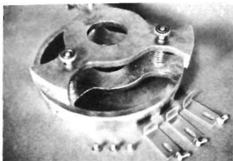
Back view of mirror mount shows tension bolts for adjusting tilt. Clips hold mirror in the mount.
