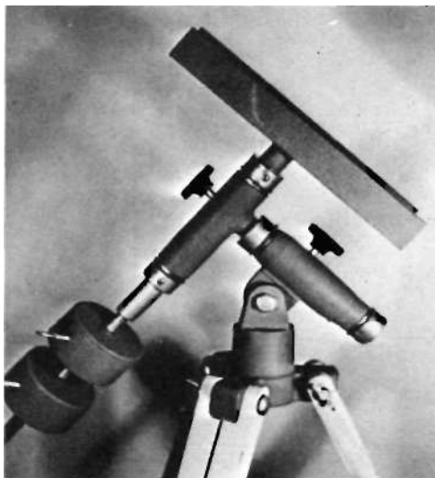
After adjustment, balancing weights are attached to the declination axis shaft on the equatorial.
