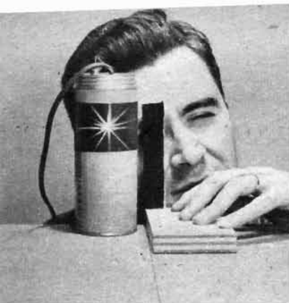
HOW THE PIN-HOLE LAMP and knife edge are used to check the curve of the mirror as it approaches a parabola. Constant testing is most important to avoid getting too deep a curve. Photograph above shows the parts of the mounting.
