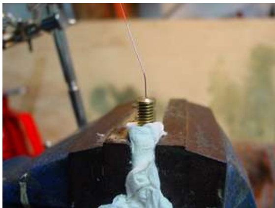
Illustration 8 Aligning nichrome with the 1mm hole
