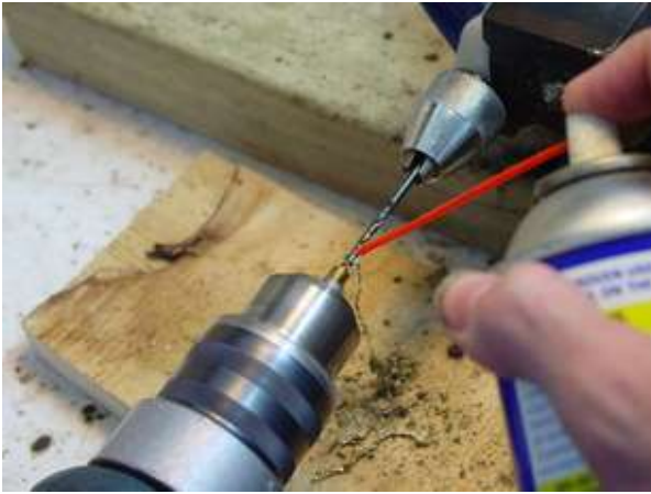
Illustration 5 Applying lubricant to the centre drilling process
