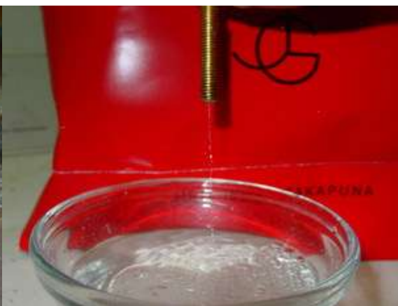
Illustration 10 Testing the nozzle with water.
