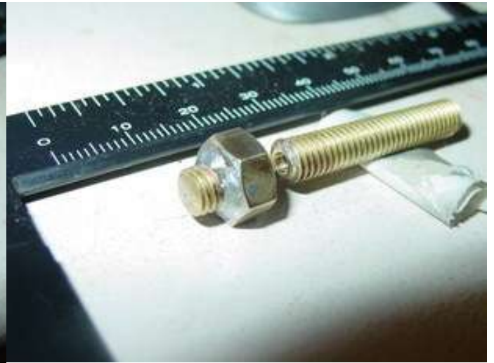
Illustration 7 The completed removable nozzle.
