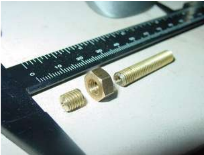
Illustration 6 The machined components for a nozzle.
