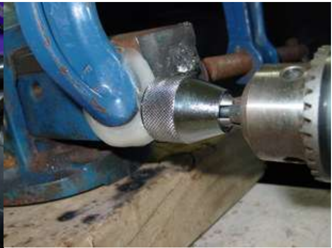
Illustration 2 First attempt, showing Polymorph far too close to the spare chuck.
