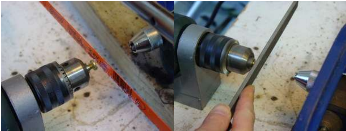
Illustration 3 Cutting off the head of the bolt.
