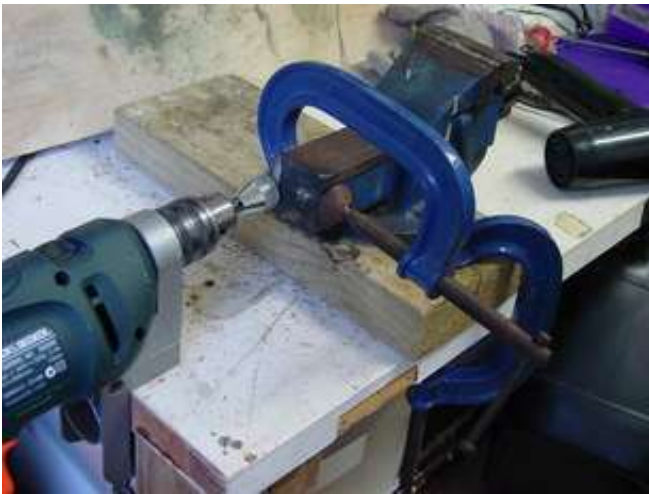
Illustration 1 Setting up lathe with both chucks gripping the smooth rod.
