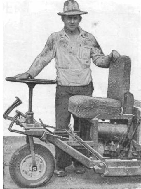
As you see here, the truck has a comfortable spring cushioned seat mounted on an angle-iron frame
