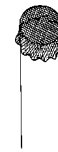
If the wire screen breaks or comes off the pipe, replace it at once.
