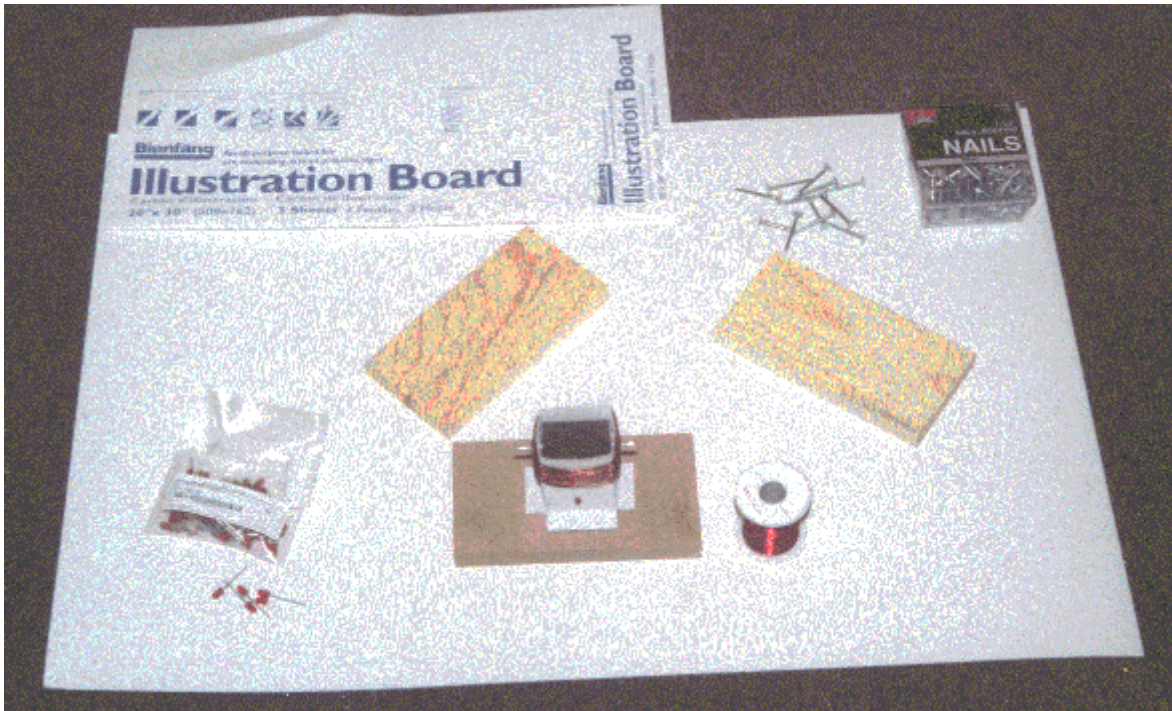
Figure 14. Construction Materials for the Alternator with a Finished Alternator
