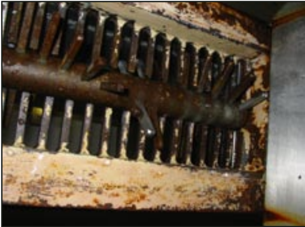
Examples of rust in the make and curing rooms.
