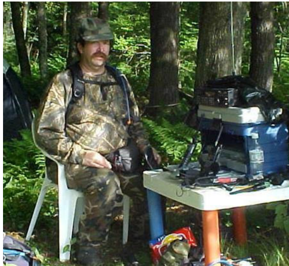
Top- This is the portable station, 2 VHF walkie - talkies, Bearcat 850 XLT scanner, various patch cables, mikes, adapters etc. Bottom - Gary L. operating the portable com satation.
