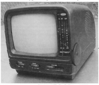
B/W portable TV with a 5 inch screen. Besides it's small size, this type of TV is a good choice for this type of monitoring as it can be operated on 12 volts directly from a vehicle, or on it's own internal battery pack as well. This particular set also includes an "A/V" (external Audio and Video) input connector which permits it to be used as a video monitor as well.
